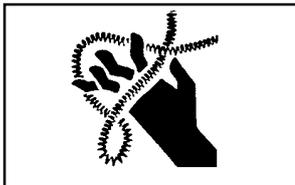
**Never grasp a rotating cable with a rag or loose fitting cloth glove that may become wrapped around the cable causing serious injury.**
