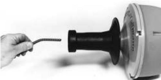
Figure 11 – Loading Loose Cable Into Canister
