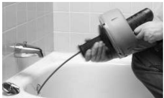
**Figure 5 – Pull Hand Grip Rearward To Engage Clutch**
