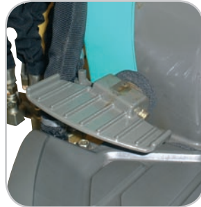
Retractable pedals (PTO pedal and swing control pedal)
