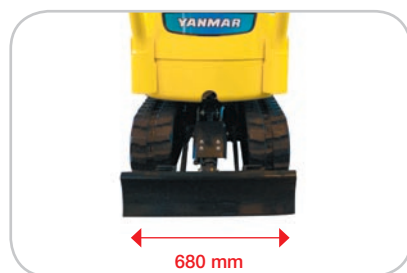
Retracted undercarriage to allow easier manoeuvre
