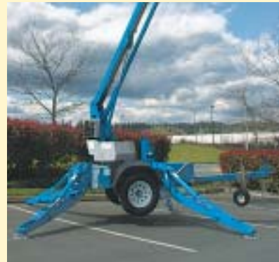
Hydraulic Outriggers with Automatic Leveling System
