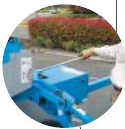
Emergency Pump Down
